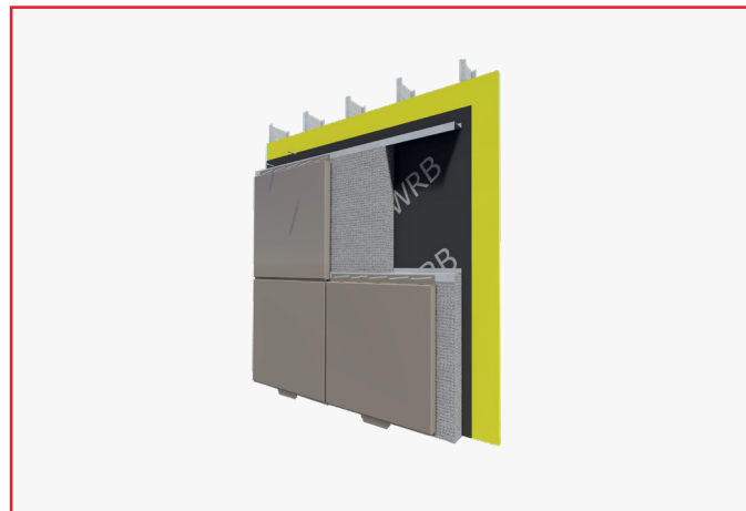
Z CHANNEL OVER EXTERIOR BATT INSTALLATION
