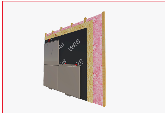
DIRECT MOUNT OVER WOOD FRAMING & SHEATHING
