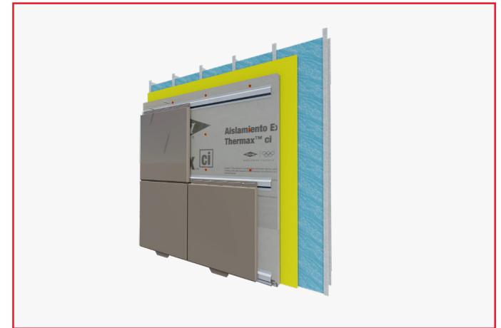
HAT CHANNEL OVER EXTERIOR INSTALLATION
